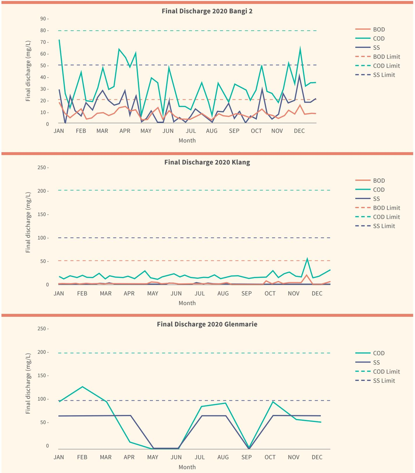
Monthly discharge at Glenmarie fluctuates widely because effluents are treated only when a certain volume is collected, as opposed to continuously. Because of the batch method used, the COD limit for Glenmarie is 200mg/L. For the year, all our plants met the relevant regulatory limits for effluent discharge.
